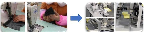
Feeding stitching + folding fixing + flipping receiving material is completed automatically
