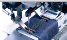
Sewing time is accelerated to 1.2 seconds/belt loop (28 stitches)
